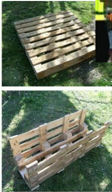
3. Fit the two end pieces to the middle part of the pallet. Screw in from the other side of the bottom piece.
